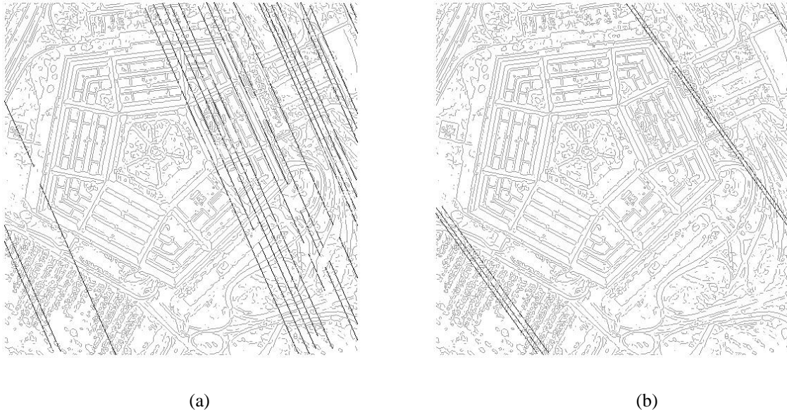
Figure 9: Lines corresponding to one \theta . In (a) \theta is 25^\circ . Lines corresponding to the 18 values in figure 8a are plotted. The lowest p index 15 corresponds to the upper left line. The lines drawn for p indices 195, 220 and 224 (lower left three lines) does not correspond to actual lines. Generally the lines plotted have quite different support, the least support for the lines in the upper left and lower right corners. In (b) \theta is 36^\circ . Lines corresponding to the 6 values in figure 8b are plotted. The lowest p index 14 is the upper left line. None of these lines correspond to actual lines.
