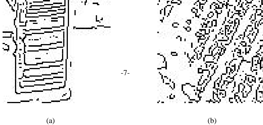
Figure 6: Edge detector behaviour. (a) is a part of figure 1b, and (b) is taken from figure 1c. Edge points forming lines are surrounded by non-edge ("white") pixels. Even in textured regions with no obvious lines, clusters of edge points tend to be surrounded by non-edge bands.
