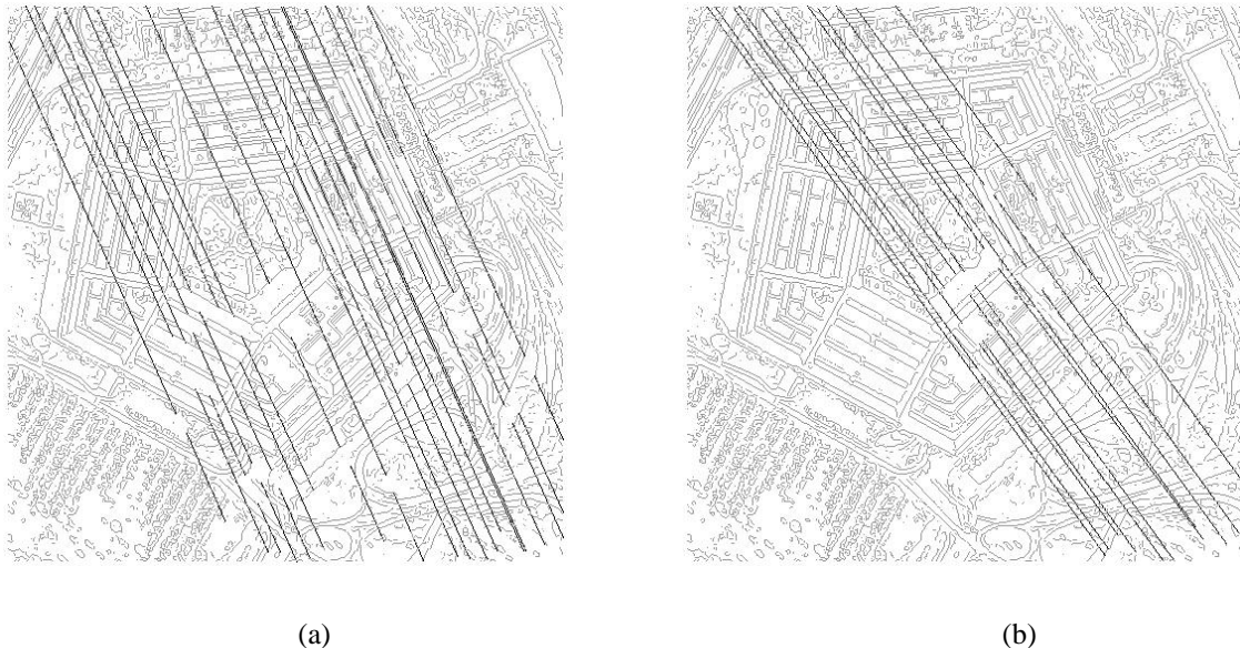
Figure 5: Lines corresponding to one \theta . The lines have been plotted with a program which produces line segments instead of lines going between images borders. In (a) \theta is 25^\circ . Lines corresponding to the 20 largest values are plotted. The lowest p index 68 corresponds to the upper left line. The lines have all approximately the same support. In (b) \theta is 36^\circ , and the 11 largest values plotted. The lowest p index 94 is in the upper left.
