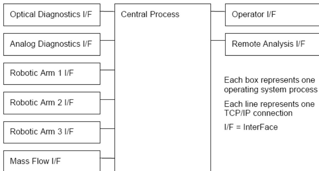
**Figure 7: Management Unit top level architecture**
